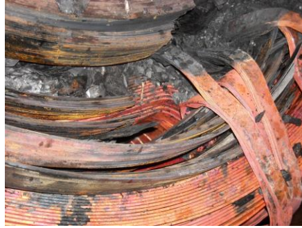
Figure 3 – Observed Winding Movement LV Winding Phase B
