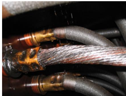
Figure 5 - Overheating of Connection #7
