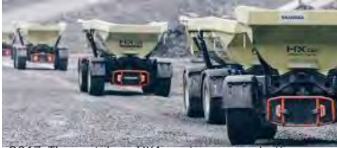
2017: The prototype HX1 - autonomous, battery electric, load carrier
