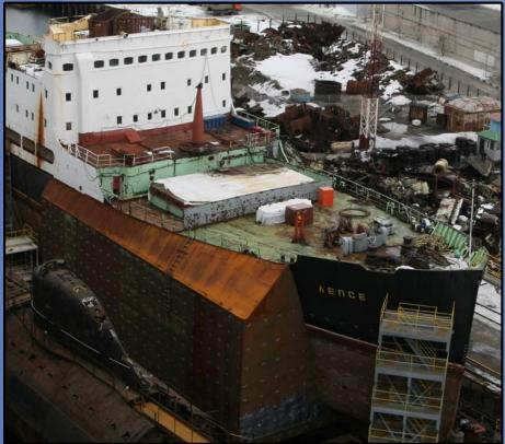
NDEP grant support: €53 million The ship has been completely dismantled, spent nuclear fuel safely packaged. Shelter has been built over the LSP and first transportation to Mayak to start in first half of 2019.
