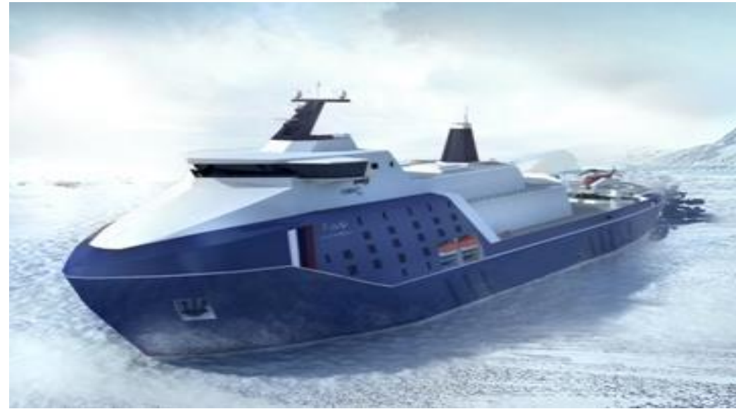
Atomic turbo-electric icebreaker Project 105010 (IB Leader) with the propulsion power of 120 MW
